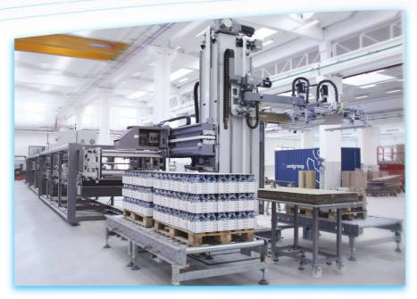
the compact design of the APS PLUS systems is the option of concentrating the use of forklifts, transpallets, etc. in a well-defined zone, optimising the management of the loading and unloading areas. The pallets and interlayers are handled on the same side of the palletiser; this does not interfere with the other activities of the production line.
