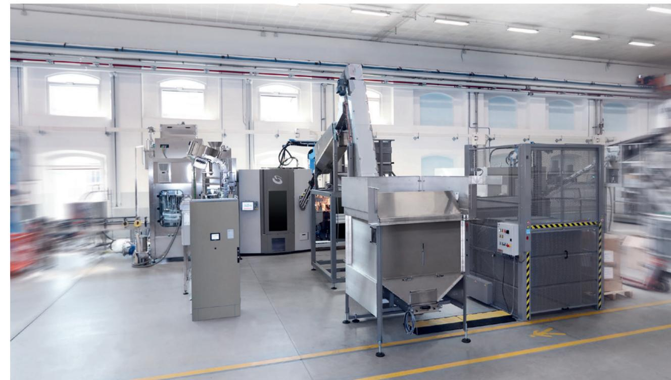
an electronic filling and capping module and shows no significant restrictions in terms of quality, safety and workability.
